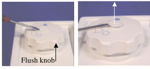
Place flat screwdriver under the small plastic insert, which is in the middle of the flush knob, and take it off.
