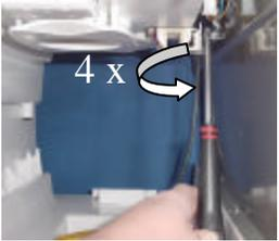
Remove the four screws located on the mechanism, allowing it to drop down.
