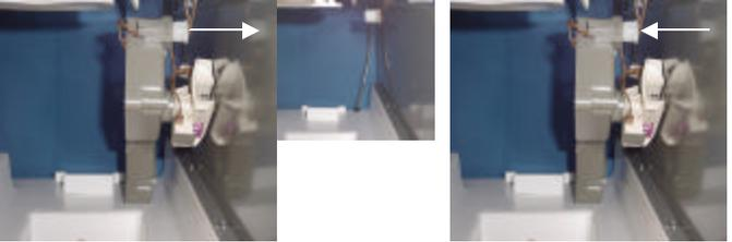
Pull the white connector loose from the mechanism, and press the connector into the new mechanism.
