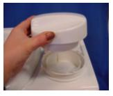
B. Push cylinder (2) down and turn it to the left to take it out. After this, the bellow cap (3) and housing (4) can be taken out.
