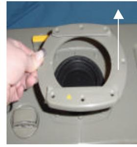
B. Ensure the two cut outs ( ) on the seal face upwards and line up with the two centre screws of the three positioned on either side of the seal cover.
