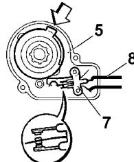
7. Screw the cover back on again or press it on, and insert the pressure rod.
