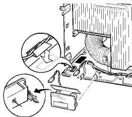
15. Plug the adapter cable onto the automatic ignition device from the rear (no need to pay particular attention to polarity).
