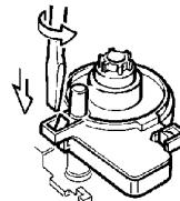
5. Use a knife, saw, or side-cutting pliers to cut an opening in the cover for passing the cable through.
