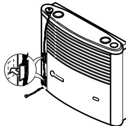
14. Use adhesive to attach another cable securing element to the base.
