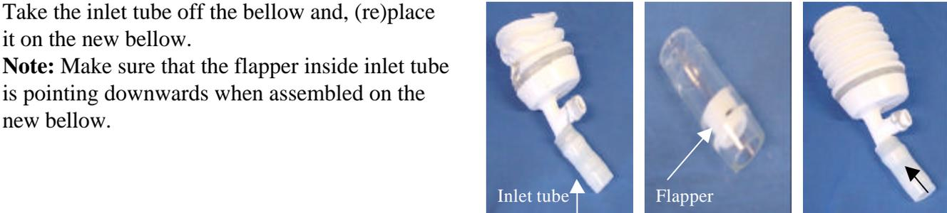
Take the inlet tube off the bellow and, (re)place it on the new bellow. **Note:** Make sure that the flapper inside inlet tube is pointing downwards when assembled on the new bellow.
