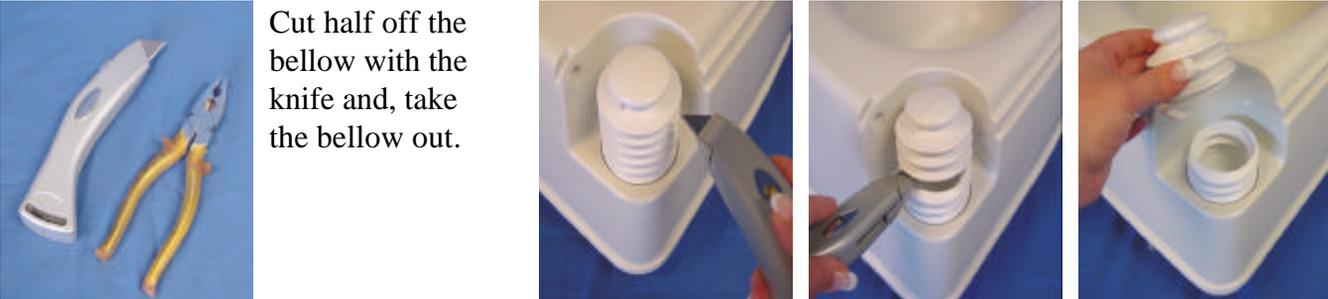
Cut half off the bellow with the knife and, take the bellow out.
