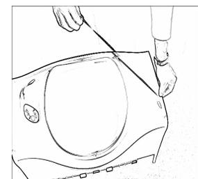
Finally, cut the seal at length
