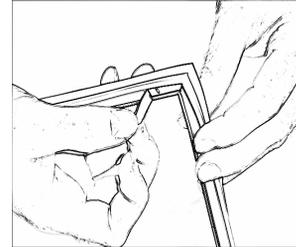
Start applying the seal first at both corners of the toilet. Then divide the remaining length along the back.
