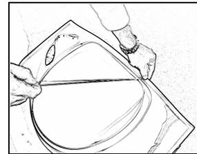
Remove the protection sheet off the tape at the left & right side of the toilet. For the sides, start removing the sheet at the free hanging end of the seal at the bottom.
