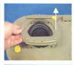
Place new lipseal C, on the waste tank. Note: Thinner flange has to face downwards towards the blade.
