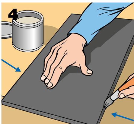
Wrap the insulation sheet around the pipe and press the glued edges together starting at the ends, then the center and then working along the rest of the length.
