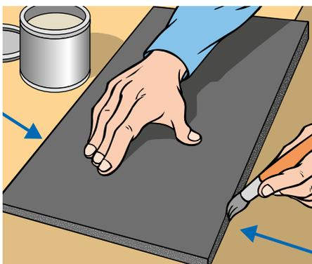
Use a straight-edged spatula to spread the glue over larger areas. If the whole of the surface is to be insulated, first apply the glue to the K-FLEX® sheet, then to the surface it is to be stuck to. When the glue has dried sufficiently, apply the sheet to the surface.
