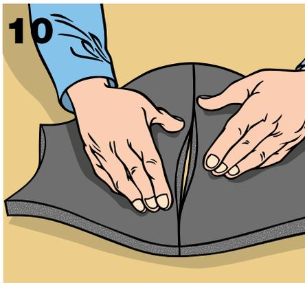
Make sure that the two sections have bonded securely on the inside as well, pressing with your fingers along the joint.
