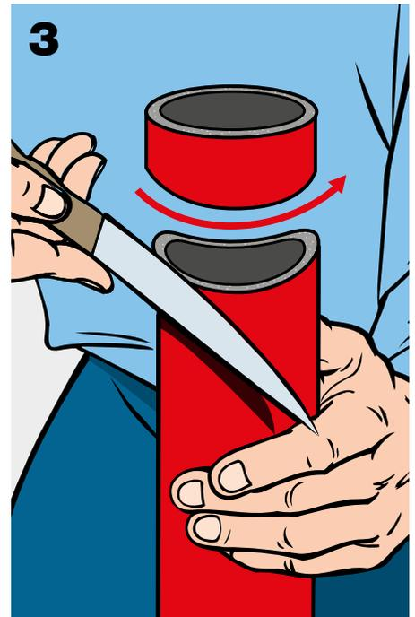
Cut the tube along its length and slide it onto the pipe so that the hole is positioned around the third pipe. Then stick the edges back together.
