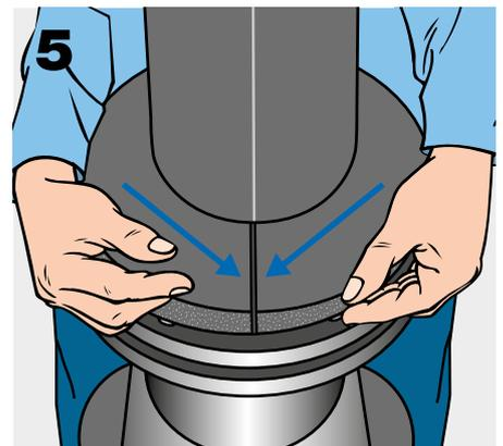
Stick the inner surfaces of the rings to the ends of the insulating tubing covering the pipes.
