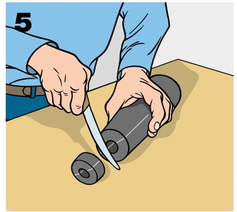
Shorten the other end, too, so that the coupling can be inserted neatly into the space left between the two existing sections.
