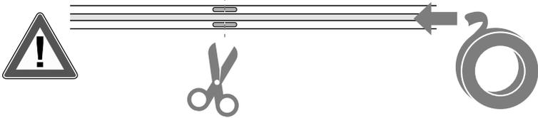
**EN** After cutting the LED strip it is advisable to tape with insulating tape the end of the strip on the cut side, otherwise the resistance to water and moisture will be lost.
