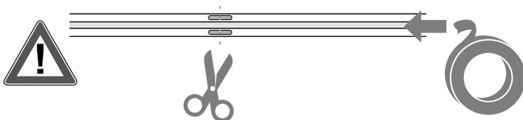
**EN** After cutting the LED strip it is advisable to tape with insulating tape the end of the strip on the cut side, otherwise the resistance to water and moisture will be lost.
